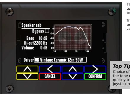
These frequency repsonses are closely matched to measurements of the devices in question in an infinite baffle.
